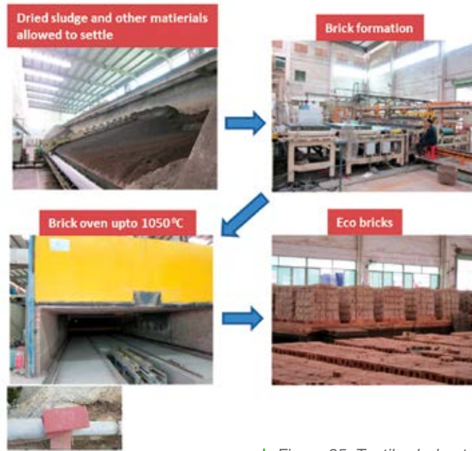
Figure 35: Textile sludge to eco-bricks facility in China
